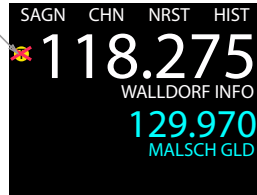
Figure 2.16.: Stuck PTT indicator
